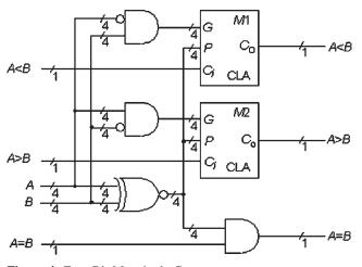
Figure 4: Four Bit Magnitude Comparator
