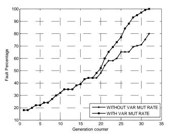
Figure 11: Effect of Changing and Not Changing Mutation Rate of Fault Detection
