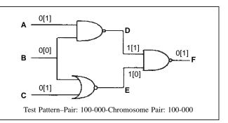
Figure 2: Test-Pattern Pair Applied to Test Circuit
